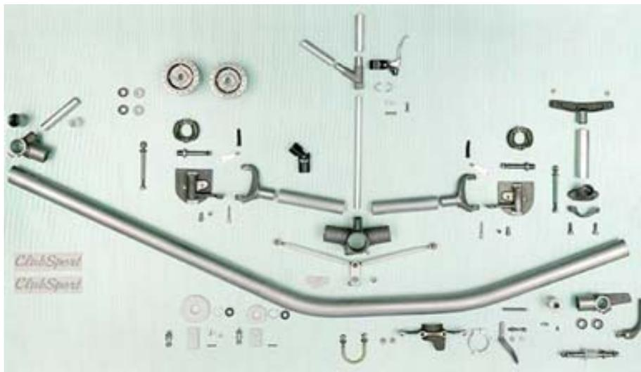
*Fig 2. Windcheetah aluminium chassis components*
